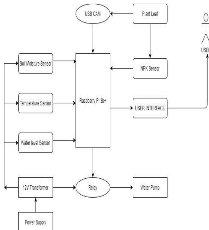
**Figure 1: Block Diagram of Working Model.**
