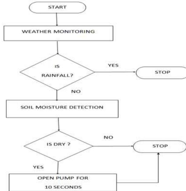
**Figure 2: Flow Chart for Automatic Irrigation System.**
