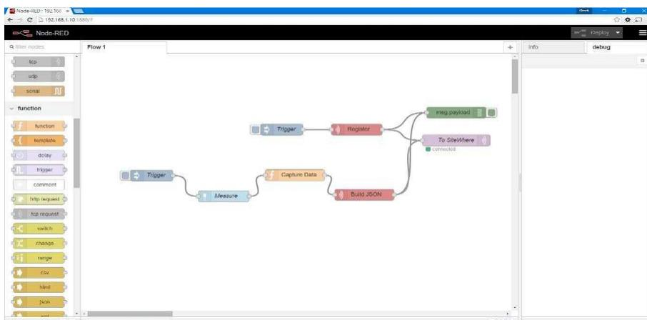
**Figure 4: Node - Red Flow for DHT 11 Sensor Dash Board.**
